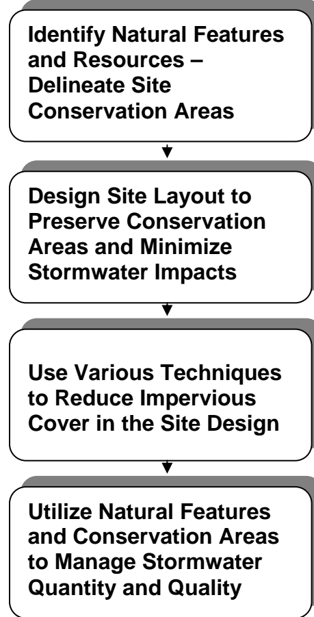
Figure 5-1. Stormwater Better Site Design Process
