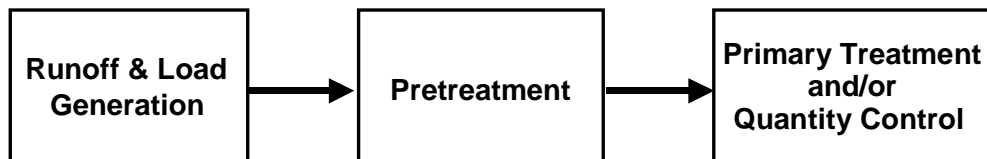
Figure 4-5. Generalized Stormwater Treatment Train
