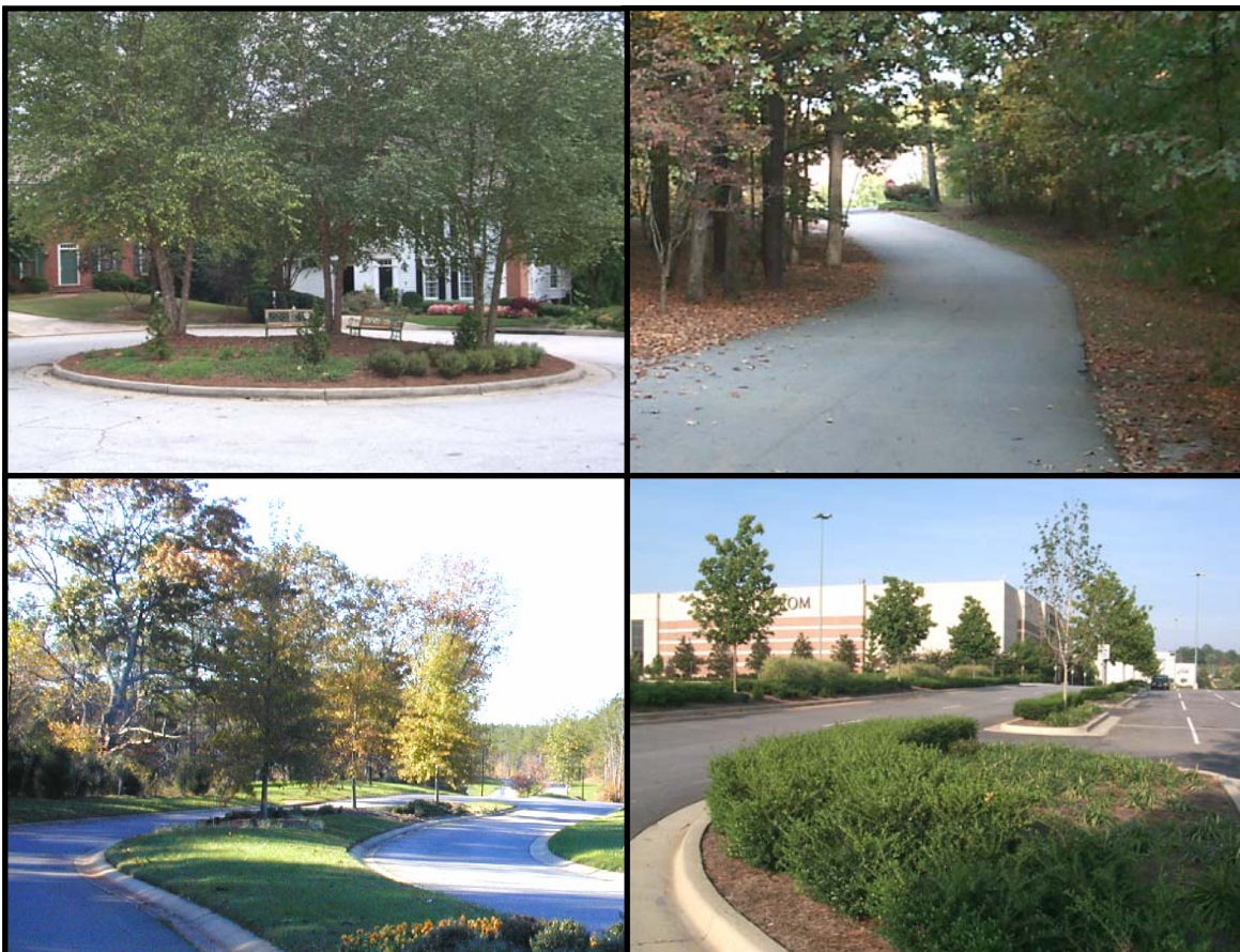
Figure 5-16. Examples (clockwise from upper left): (a) Cul-de-sac with Landscaped Island; (b) Narrower Residential Street; (c) Landscape Median in Roadway; and (d) “Green” Parking Lot with Landscaped Islands
