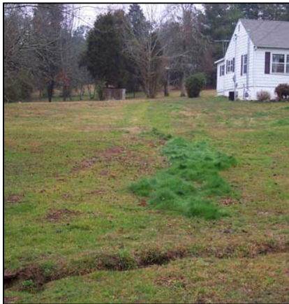
Photo 2 Sign of failed septic system
